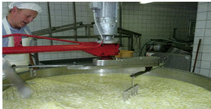
Figure 6. Cuve double paroi (pasteurisation-coagulation –tranchage) (Web 2 )
